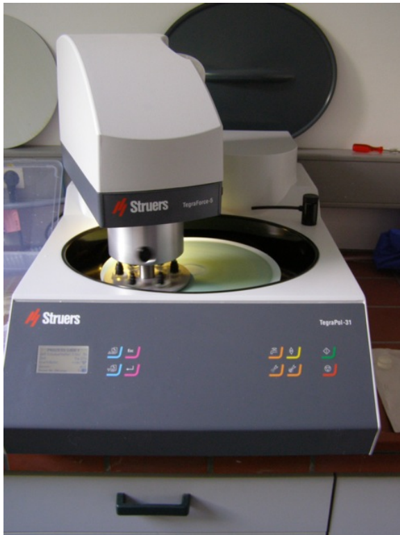
Polishing apatite and zircon mounts
